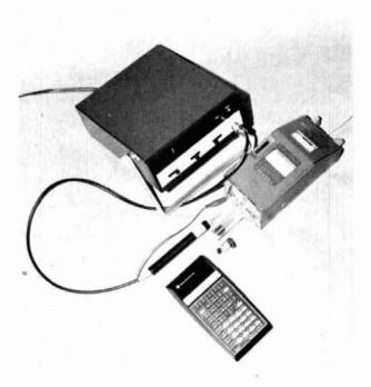
fig. 5. Setup used to speed up the inductance measurement process. The toroidal coil under test was paralleled by a known precision silver mica capacitor. The exact frequency of the circuit was read with a digital counter which measured the frequency of rf generated by the grid dip meter at resonance. All numbers were inputted to the TI-59 programmable calculator which resolved the equation for L or C.
